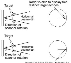
Radar cannot display targets as separate echoes because they are within the beamwidth.
